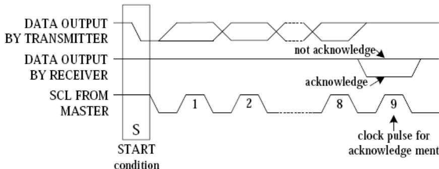
Figure 4. Acknowledgement on the 2-line Interface
